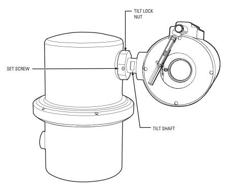
Figure 11. Set the Tilt Position
